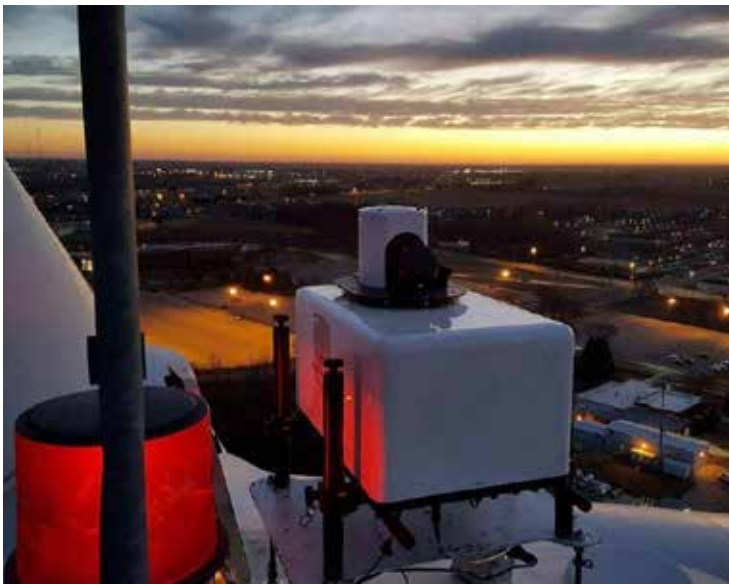
One of two Doppler wind LiDARs installed on top of the 2.5 MW Clipper wind turbine at Kirkwood Community College in Cedar Rapids, IA. LiDAR stands for Light Detection And Ranging and is an instrument used to remotely measure wind speed up to 3 km ahead of and in the wake of wind turbines. (see page 8). Photo: Corey Markfort .
