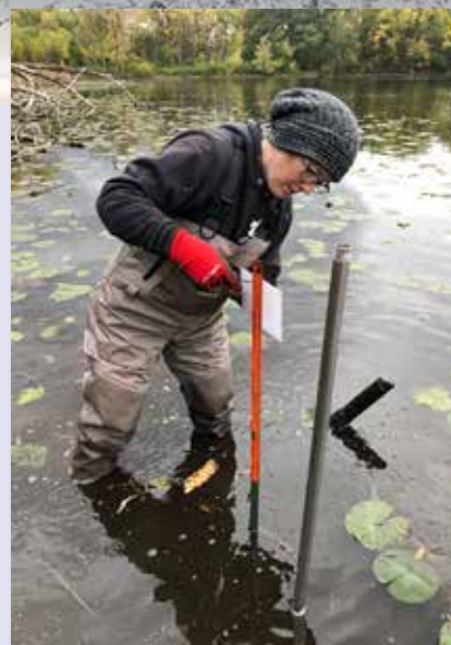
Jessica Meyer installs a piezometer in a lakebed. The piezometer is a small diameter well that will provide data to constrain the direction of water flow and the associated iron mass discharge between the lake and the underlying aquifer.
