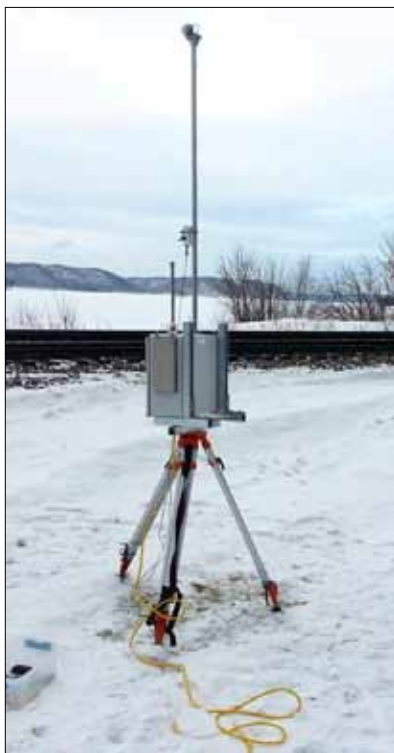
A device monitors air quality next to a rail line that carries silica sand for frac mining.
