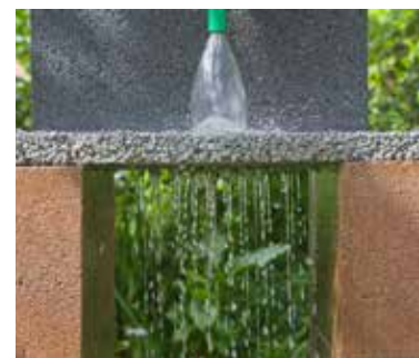
Water can be seen passing through cement in this permeable paving demonstration.
