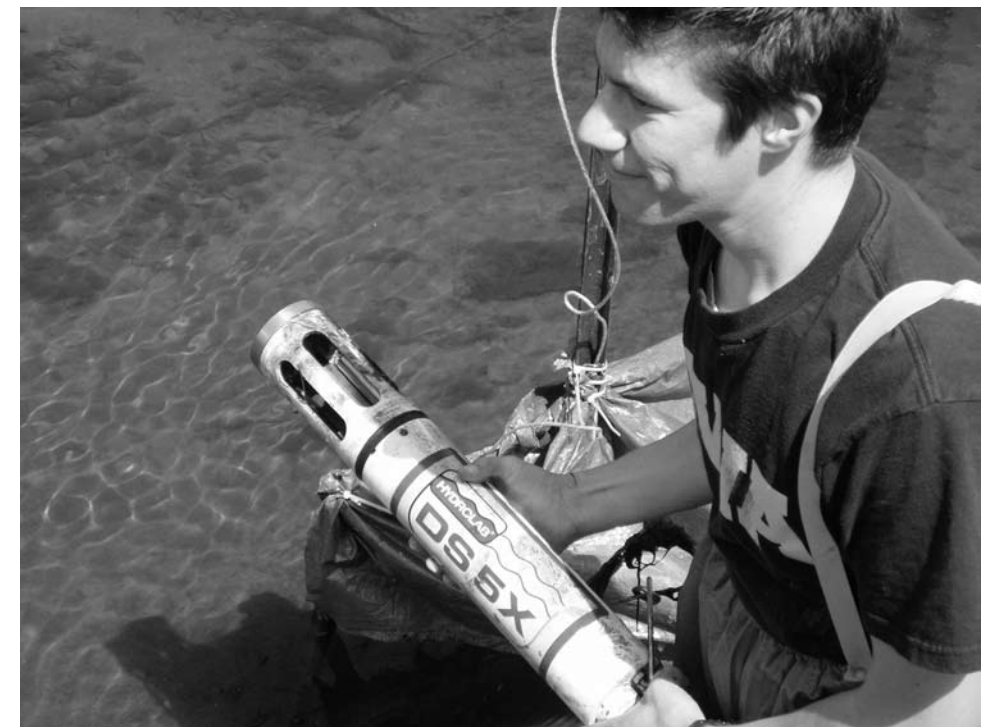
Graduate student JV Loperfido, sampling in the WATERS Clear Creek test bed, inspects an in-stream water quality monitor that operates unattended for weeks at a time.
